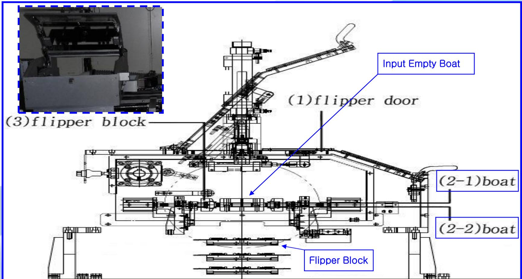
1. Input empty Boat(upside down) into Flipper System
