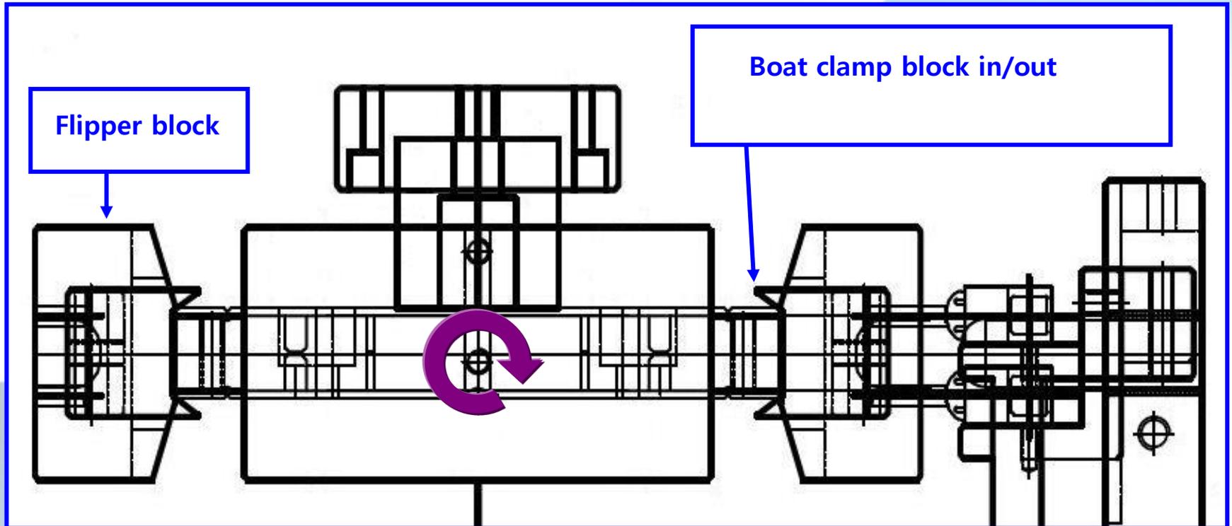
3. Flipper block clamp Top and Bottom Boat.
