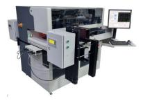
Full **Flip Chip** process capability including chip flipping, bump fluxing and chip accurate alignment over a high resolution Up Looking Camera. The machine performs cold and heated processes including:
