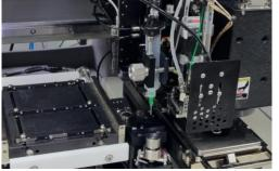
**Heated** applications up to 500°C for different **Eutectic** processes including AuSn, AuGe, AuSi and other interconnection materials.
