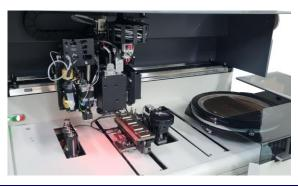
The machine features its unique **Bond Line Thickness (BLT)** control capability for Silver Glass, MEMS and wet **Die Stacking** applications.
